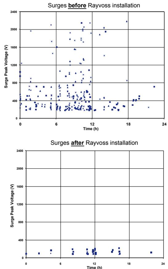
Figure 3: Power line transient overvoltages in a conveyor belt PLC measured in a 24h period before and after installing Rayvoss.
