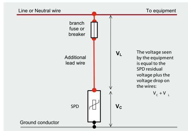
Figure 1: Residual voltage in Kelvin and T-connection applications.
