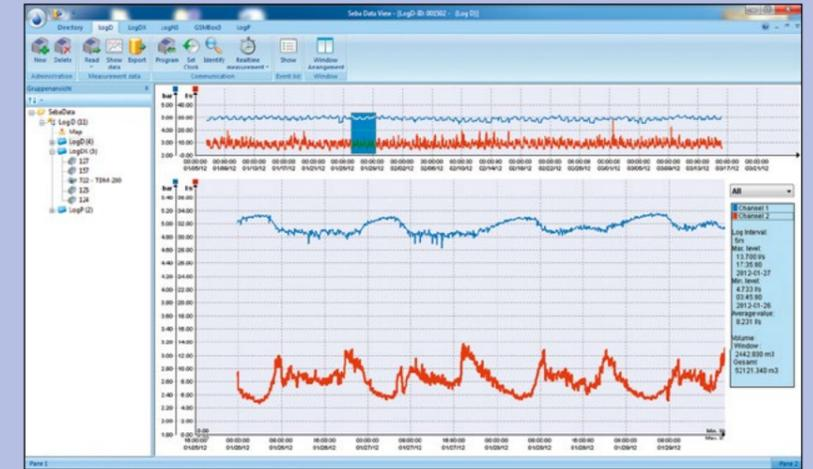
Data set of multiple days showing flow and pressure
